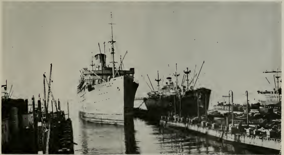
The SS Argentina, which served as a troopship during the war, enters a 25,000-ton floating drydock — the largest in the country — at the Bethlehem Brooklyn Division yard. The vessel is being reconvered for peacetime service by the U. S. Maritime Commission. By mid-summer the 587-foot, 20,614-ton ship will emerge again as a luxury liner, to be operated on the "Good Neighbor" run to east coast South American ports by the Moore-McCormack Lines.
